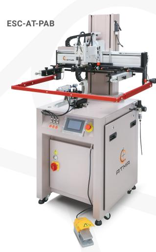
Precision screen printing machine for all-purpose printing on small-sized flat and cylindrical substrates with high register accuracy up to a material thickness of 260 mm. Also available in version ESC-AT PA for flat printing and as ESC-AT PB for printing on moulded substrates in cylindrical, conical and oval shape.
